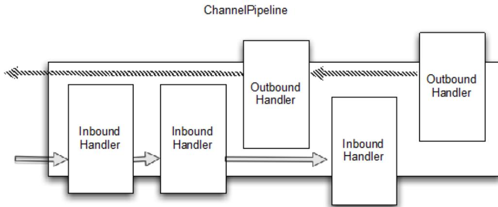
Figure 6.1 `ChannelPipeline`
