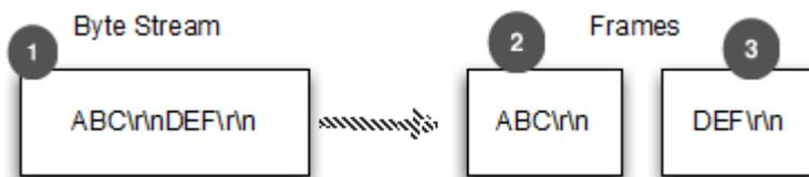
Figure 8.5 Delimiter terminated frame handling
