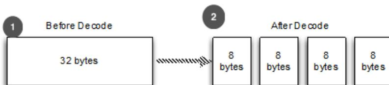
Figure 8.6 Message of fixed size of 8 bytes
