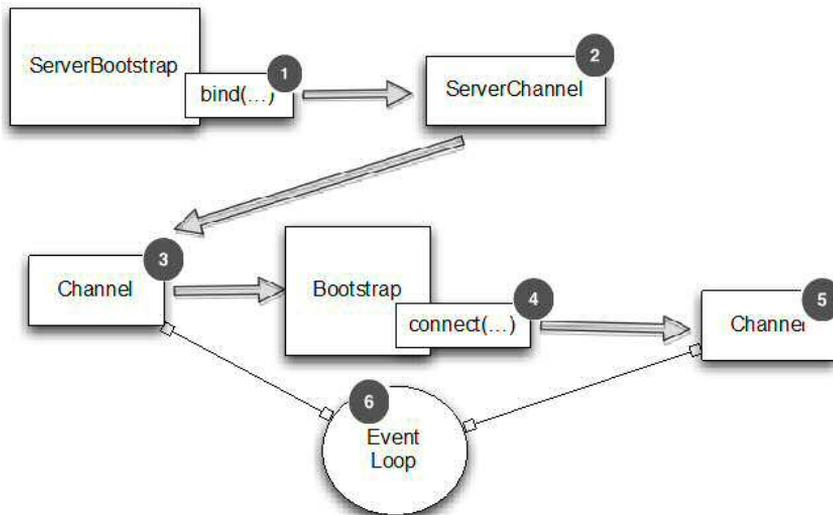
Figure 9.4 Share EventLoop between channels with ServerBootstrap and Bootstrap
