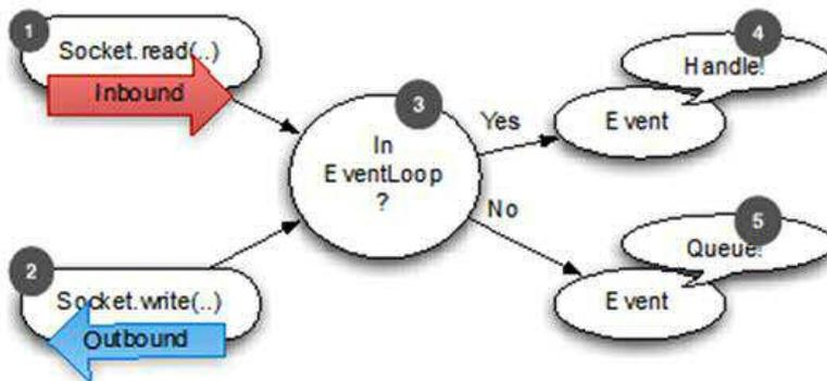
Figure 15.3 EventLoop handling of reads and writes
